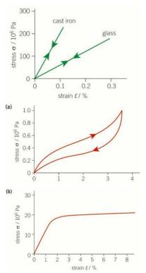
For a brittle material like glass, elastic behavior is shown until the breakpoint where the material snaps. There **is no plastic deformation**, and the loading and unloading curve are the same.
