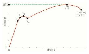
On a stress-strain graph for a wire, P is the **limit of proportionality**. Up until this point, Hooke's law is obeyed. E is the elastic limit, and beyond this point the wire will experience plastic deformation. Y1 and Y2 are yield points where there is rapid extension. UTS is the ultimate tensile strength, **the maximum breaking stress** that can be applied to the wire. Strong materials have a high UTS.
