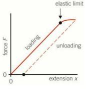
A metal wire obeys Hooke's law and shows elastic deformation until its elastic limit. The loading curve is the same as the unloading curve in this region. Beyond this point it experiences plastic deformation. The unloading curve shows how this plastic deformation leaves a permanent extension of the wire.
