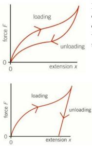
Rubber is does not experience plastic deformation, but it does not obey Hooke's law. The area between the loading and unloading curves is a **hysteresis loop**. This area represents the **energy** that was required to **stretch the material out**, which was transferred to thermal energy when the force was removed.
