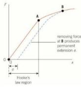
Up until point A, the force acting on the spring is proportional to the extension. The spring shows **elastic deformation**, meaning that it will return to its original shape when the force is removed. The gradient of the line here is equal to the force constant.
