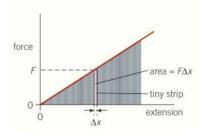
When a material is deformed elastically, **work is done**, and transferred in to the material. It is stored as **elastic potential energy**, E, and released when the material is allowed to return to its original length.
